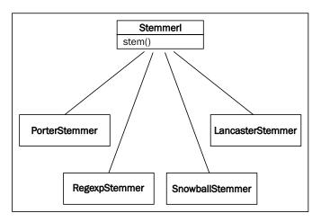
All the stemmers covered next inherit from the StemmerI interface, which defines the stem() method. The following is an inheritance diagram that explains this:
